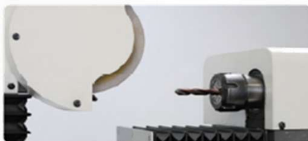
Tighten the collet with a wrench, leaving 20–30mm of the cutter exposed.
